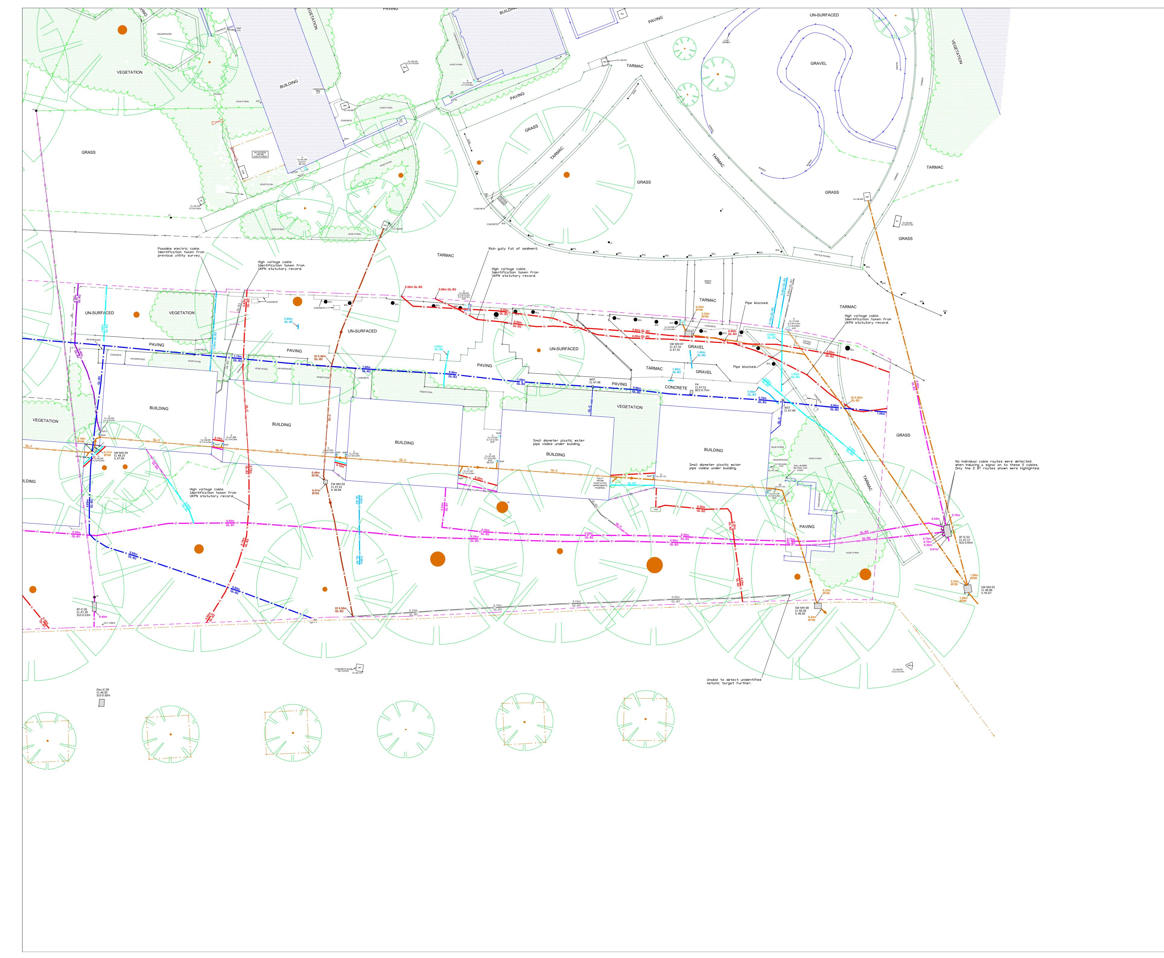
A variety of detection technologies were used to produce the underground information recorded for this non-invasive survey. Variations in ground conditions, depth and density of services and signal interference from surrounding features can affect the accuracy of these technologies, therefore 100% detection and accuracy cannot be guaranteed. All utility/service depths are in metres and are taken to the top of utility/service unless otherwise stated.
